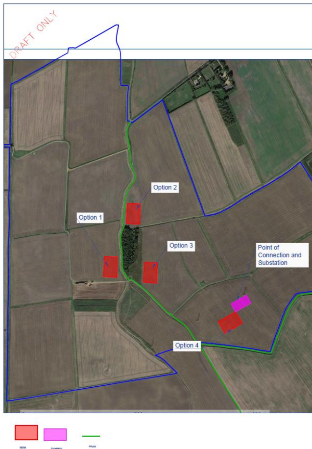
Figure 4: Optioneering exercise to determine most suitable BESS location
