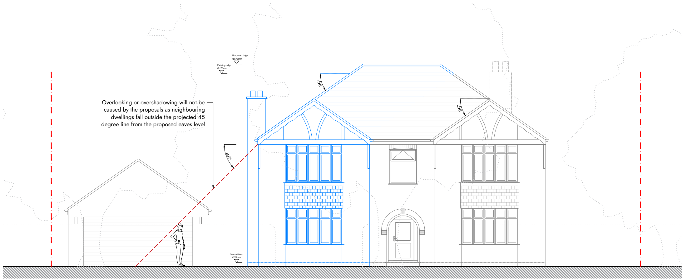
01 Daylight assessment elevation - proposed 1:100@A2
