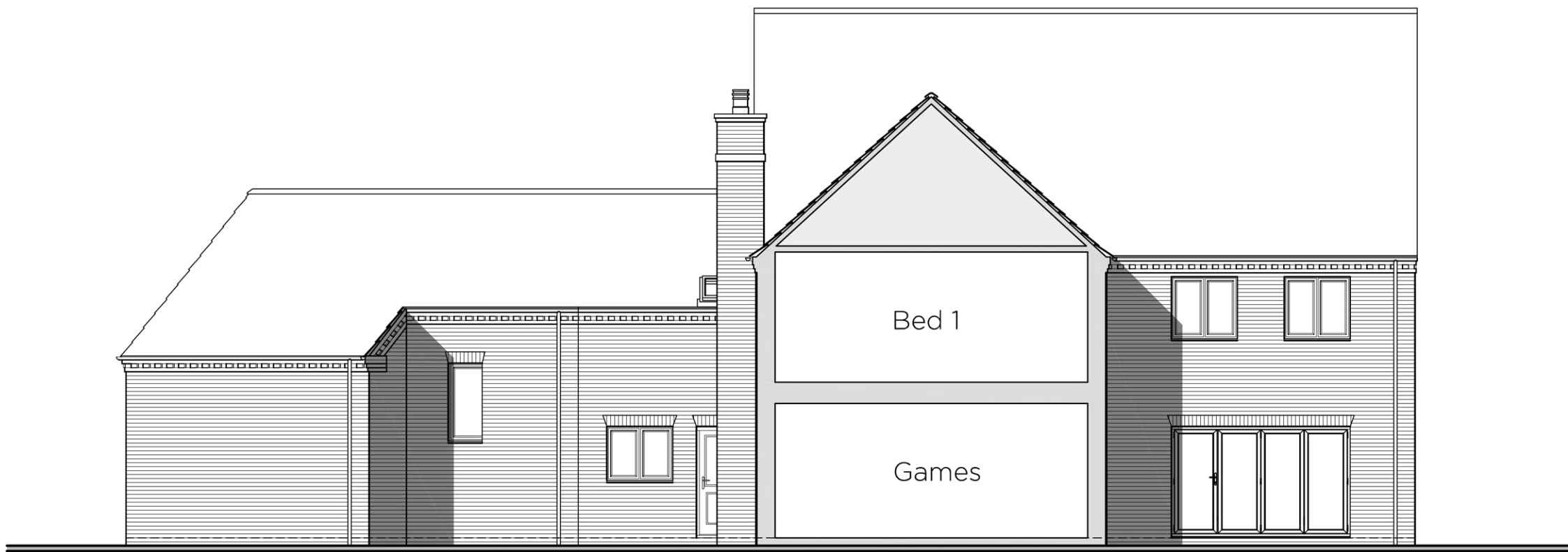
Rear Sectional Elevation (Main House)
