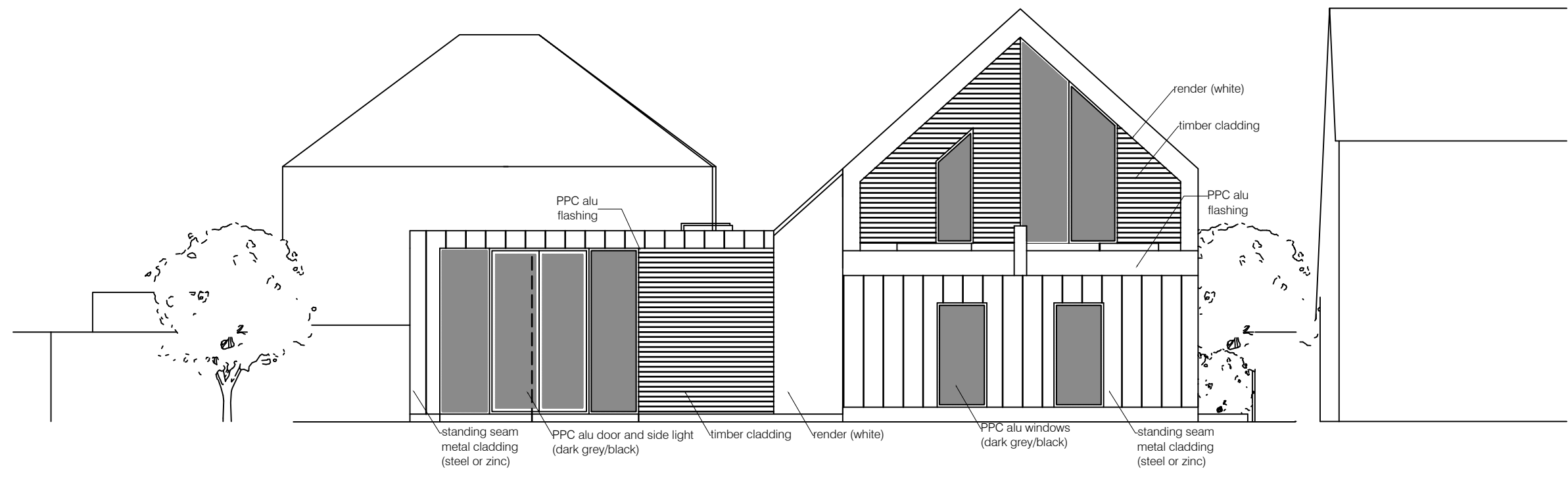
2 EAST ELEVATION 1:100 0m 0.5 1 1.5 2 3 4 5
