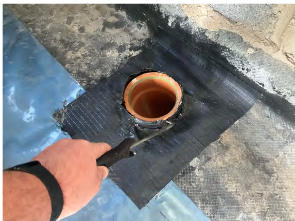
Plot 1. Probe testing to pipe penetration details.
