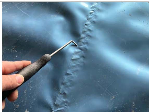
Plot 4. Probe testing along hand welded membrane lap joints.
