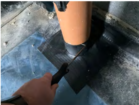
Plot 5. Probe testing to pipe penetration details.
