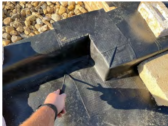
Plot 4. Probe testing to door threshold detailing.
