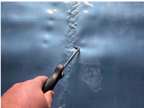
Plot 5. Probe testing along hand welded membrane lap joints.
