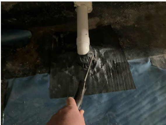
Plot 4. Probe testing to pipe penetration details.
