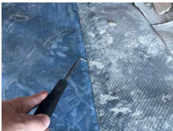
Plot 1. Probe testing along hand welded membrane lap joints.
