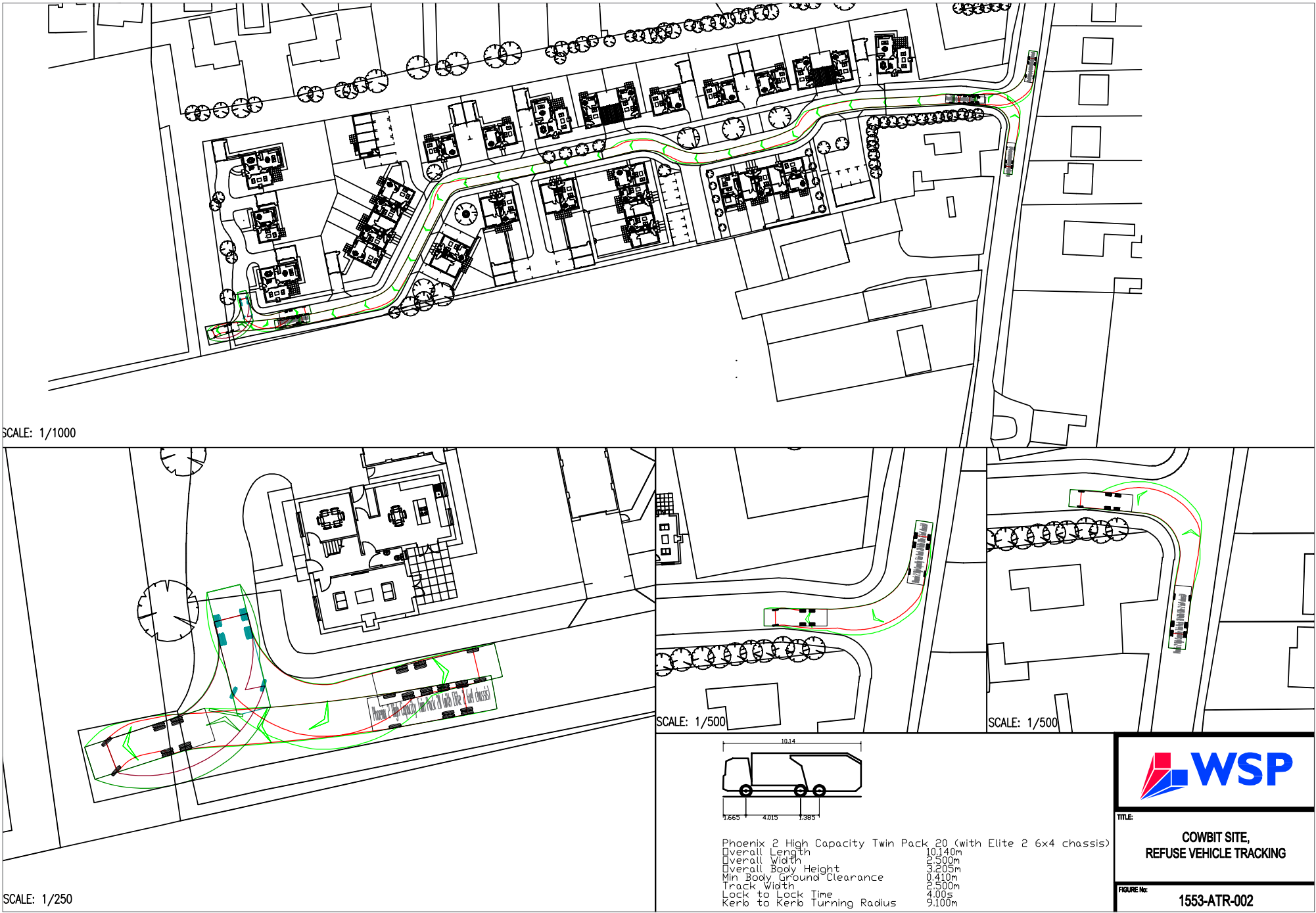
Fig. 12: Tracking diagram for refuse vehicle
