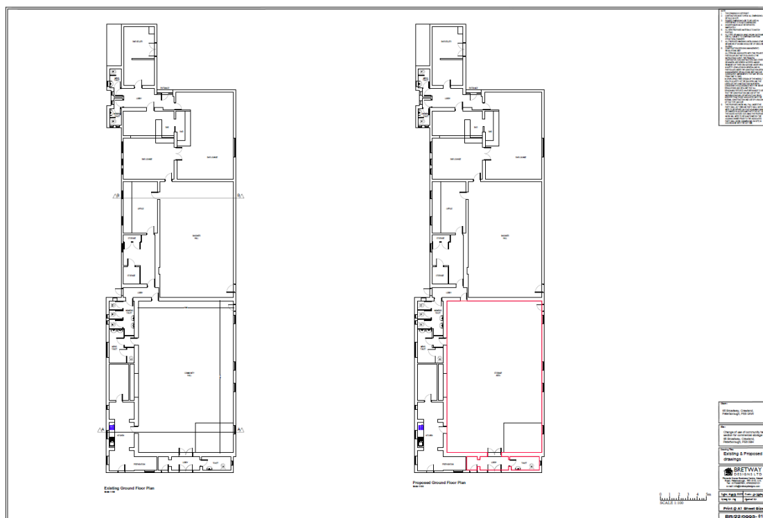
Figure 3 – Drawing showing existing and proposed sections for the change of use at 65 Broadway Crowland, PE6 0AW
