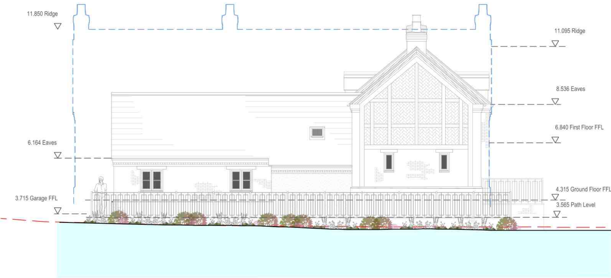
East Elevation Scale 1:100
