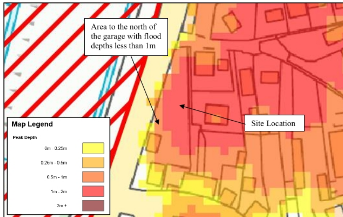
Figure 3 – SFRA 2116 Residual Peak Depth Map
