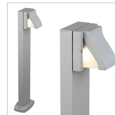
indicates 43707 Dylan LED post light Uses 36no 0.06w leds. Height 750mm Length 110mm, width 120mm. 59 Lumens output with a single 3w natural light led. Part L compliant with motion sensor. These lights are 'Bat friendly'.
