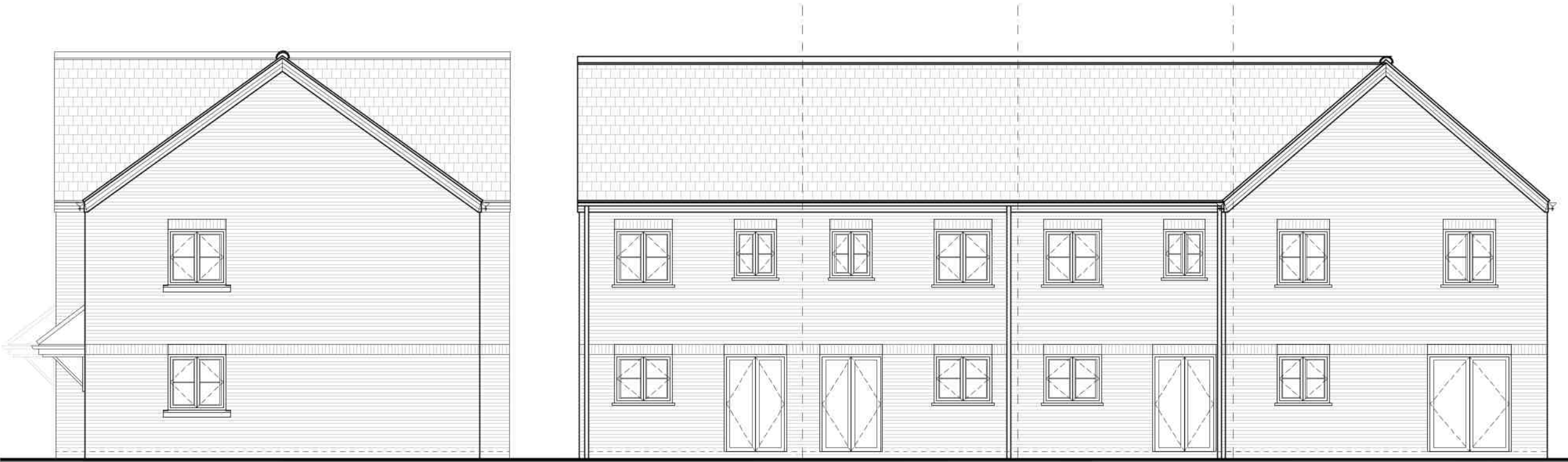
SIDE ELEVATION REAR ELEVATION
