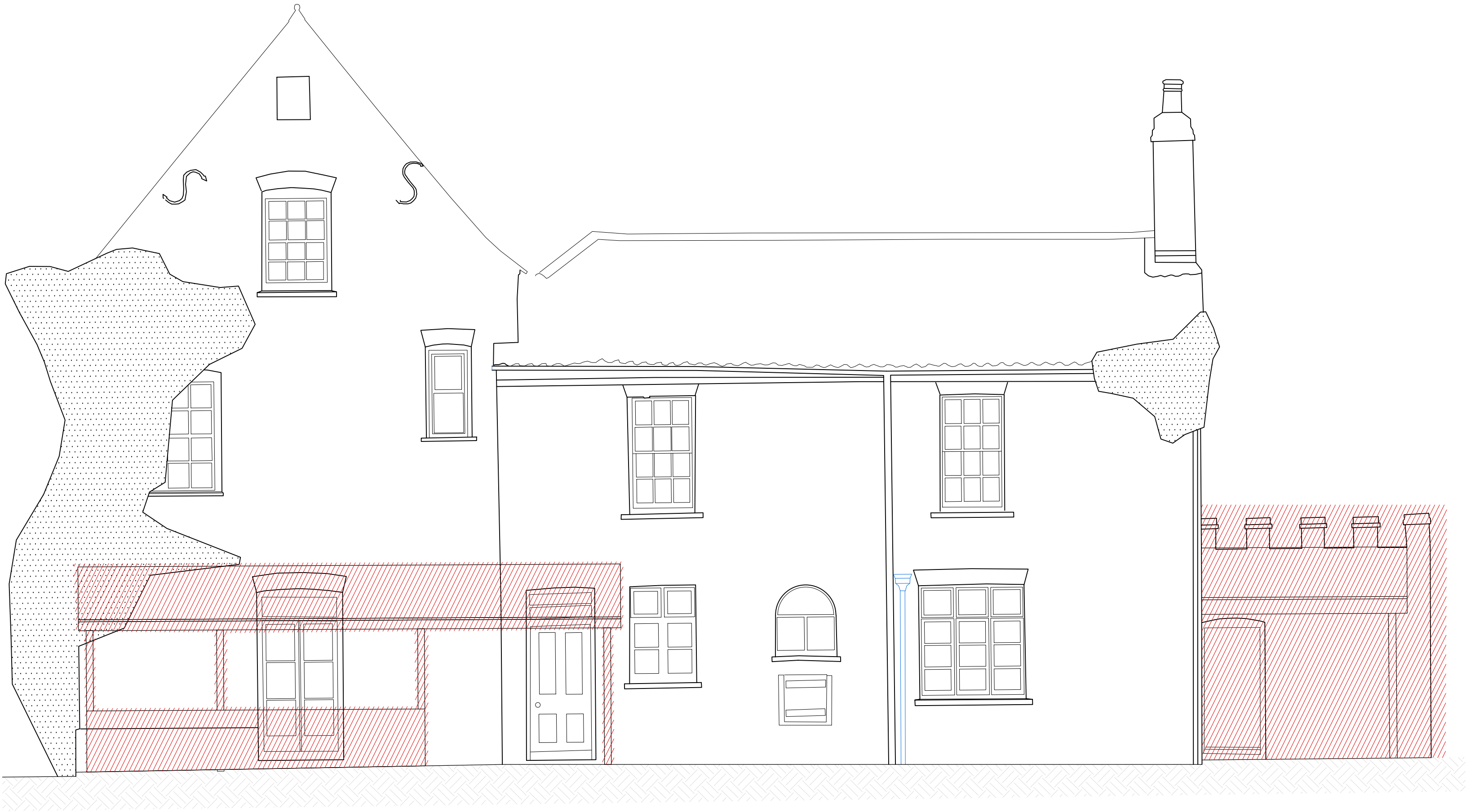
PROPOSED DEMOLITION WORKS ELEVATION A
