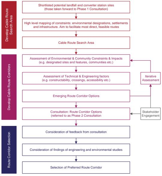
Figure 2.10 Approach to Cable Routeing
