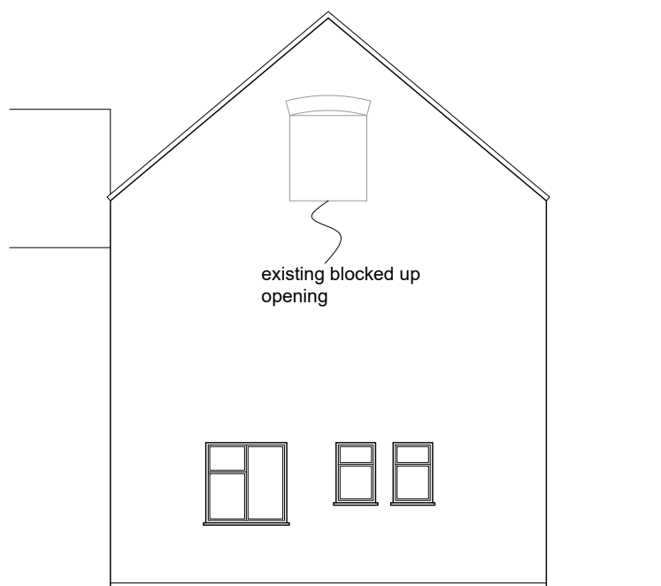
Existing Rear Elevation (1:100)
