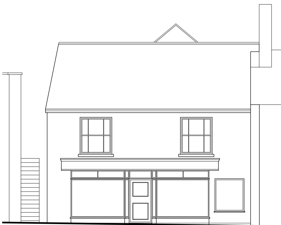
Existing Front Elevation (1:100)
