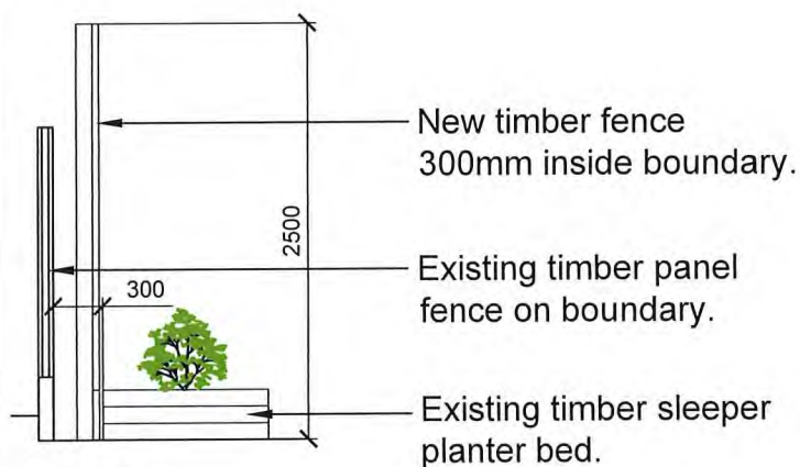
Fence In Section - As Proposed (not surveyed) Scale 1:50
