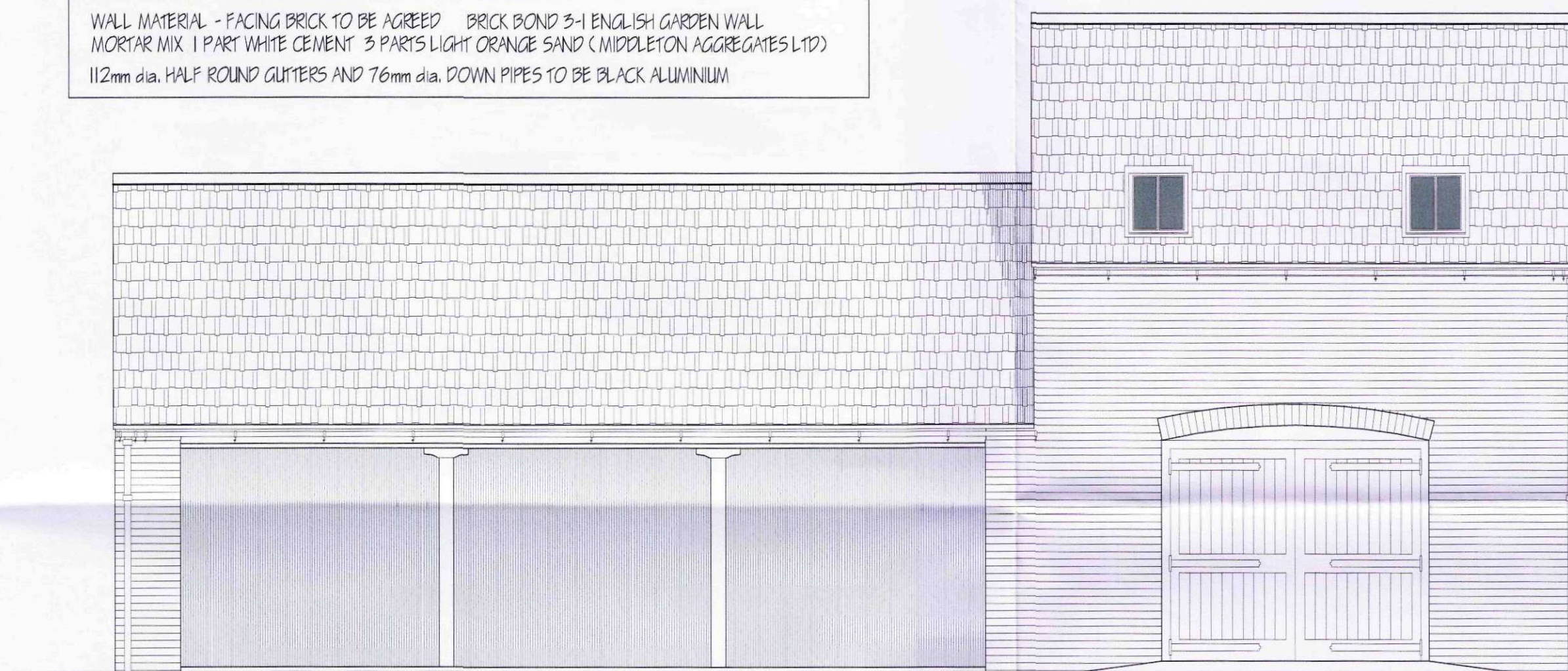
SOUTH - WEST ELEVATION
