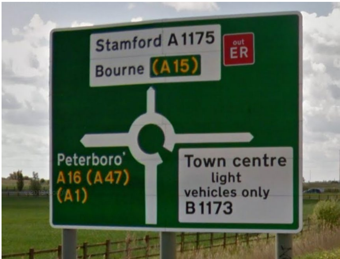
Figure 1 Example road sign indicating emergency evacuation route highlighted by red 'out ER' box. Image capture: May 2019 © Google
