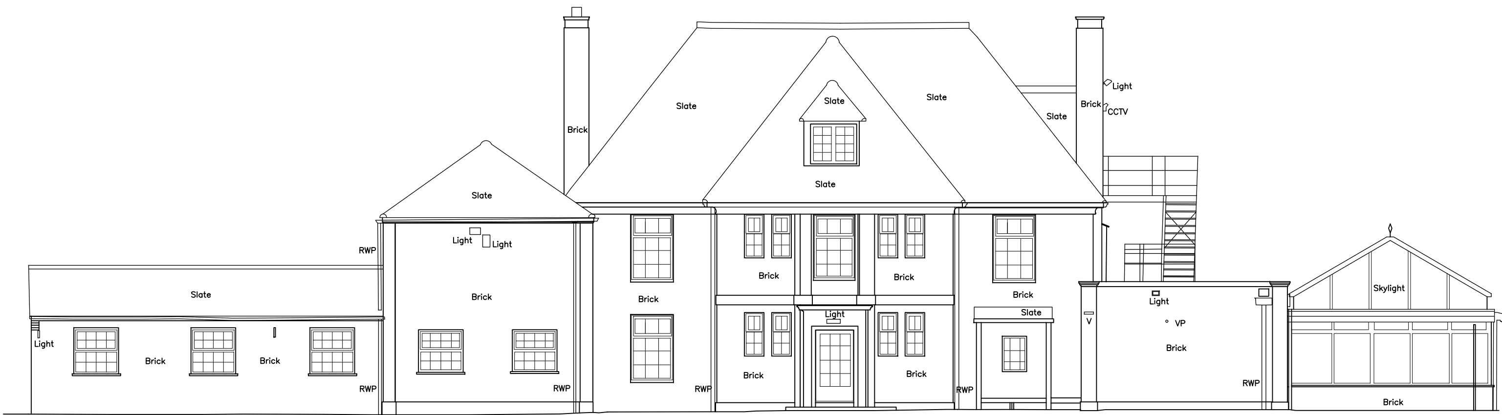
Existing North West Elevation ( Elevation 5 )
