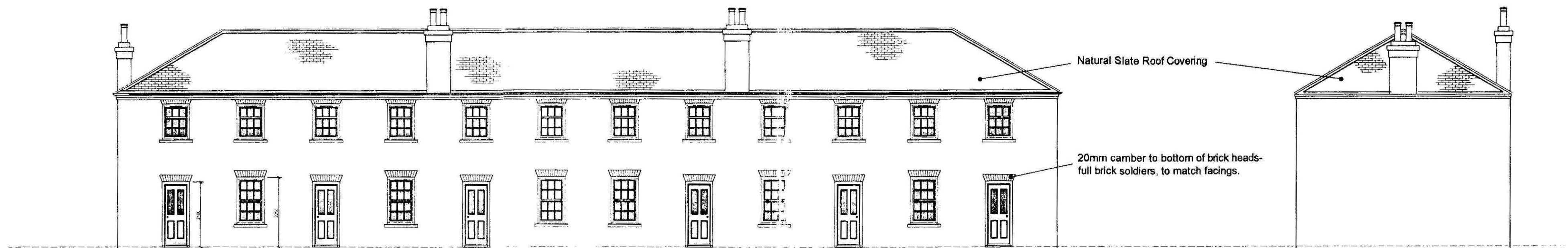
WEST ELEVATION - TO REAR GARDEN AREA
