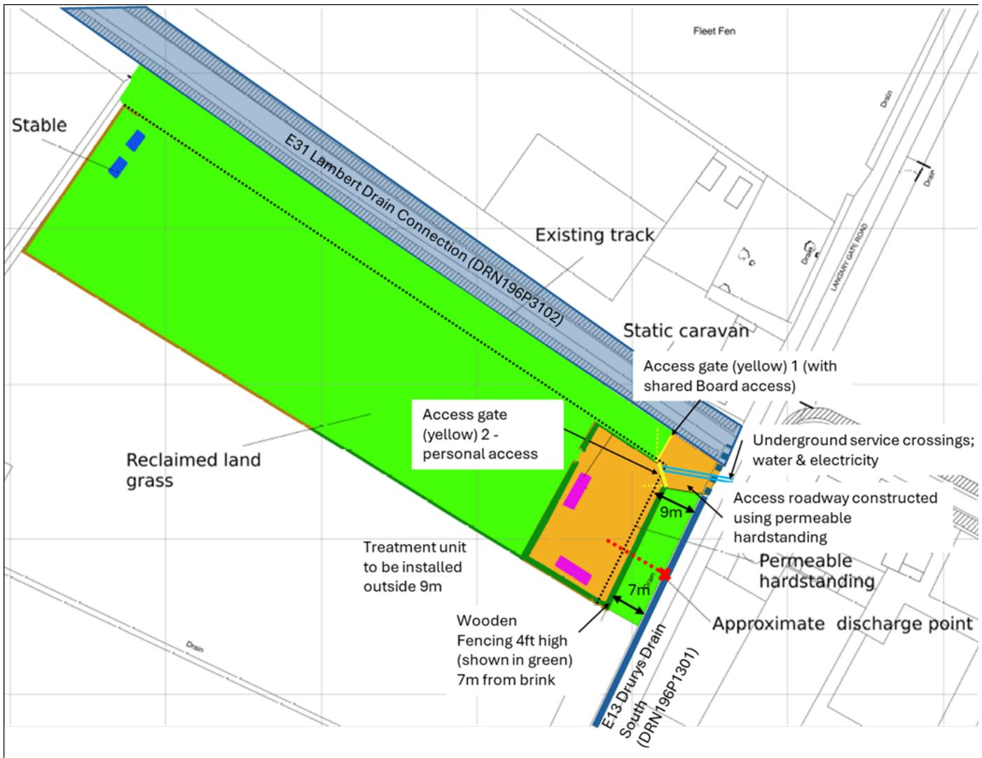
Drawing showing Board arterial watercourses in blue, treated foul water discharge point, location of new fencing, gates, underground services and access roadway material. The fencing, access roadway, services may continue west, however, consent is only for the works within 9m of the Board arterial watercourse as shown by the dashed black lines. Base drawing supplied by agent (17/04/2025) additional annotations carried out by Board (04/06/2025).
