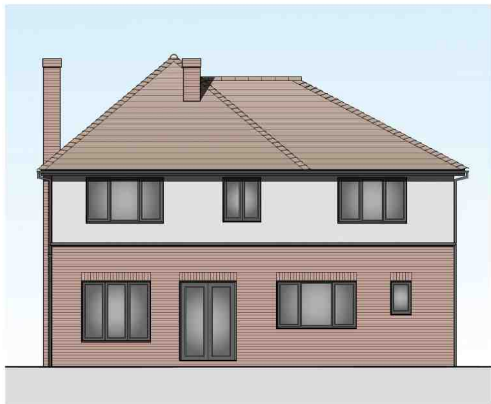
Proposed Rear (E) Elevation Scale 1:100
