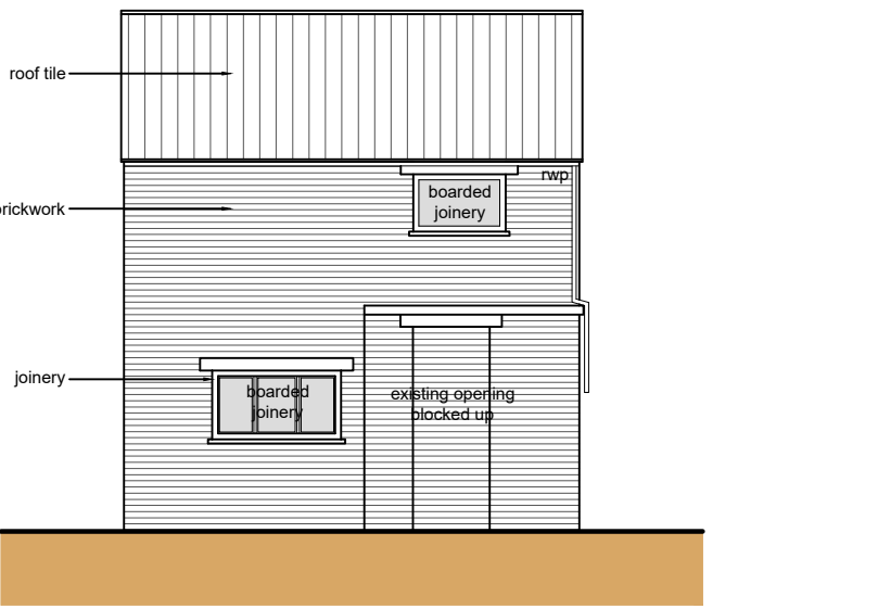
Rear Elevation (W)
