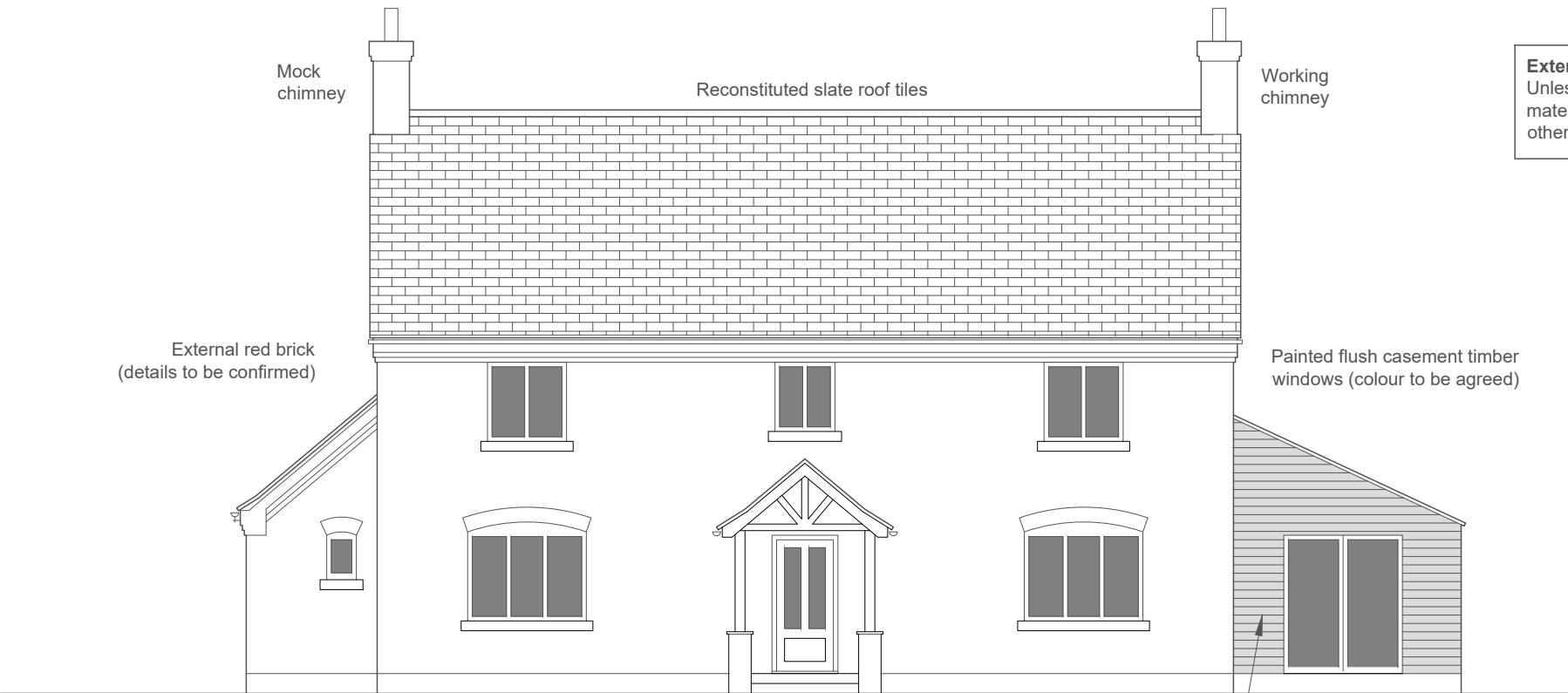
North West Elevation (front)
