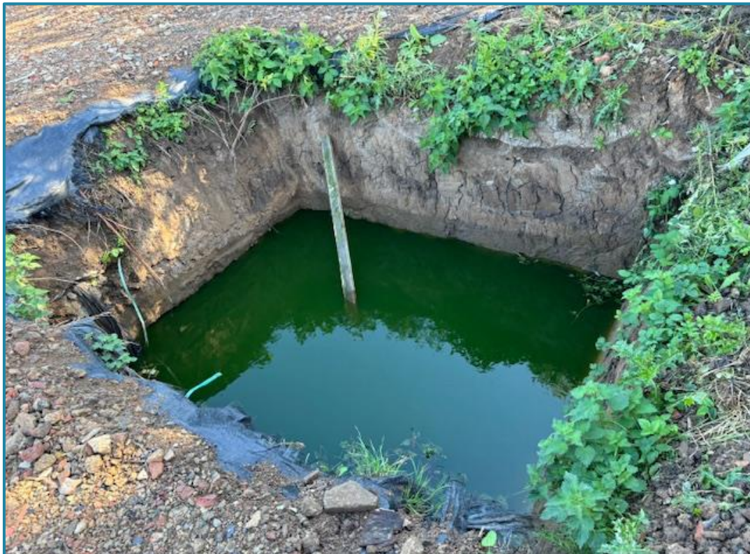
Photo 4.1 – Percolation Test (TP 02)
