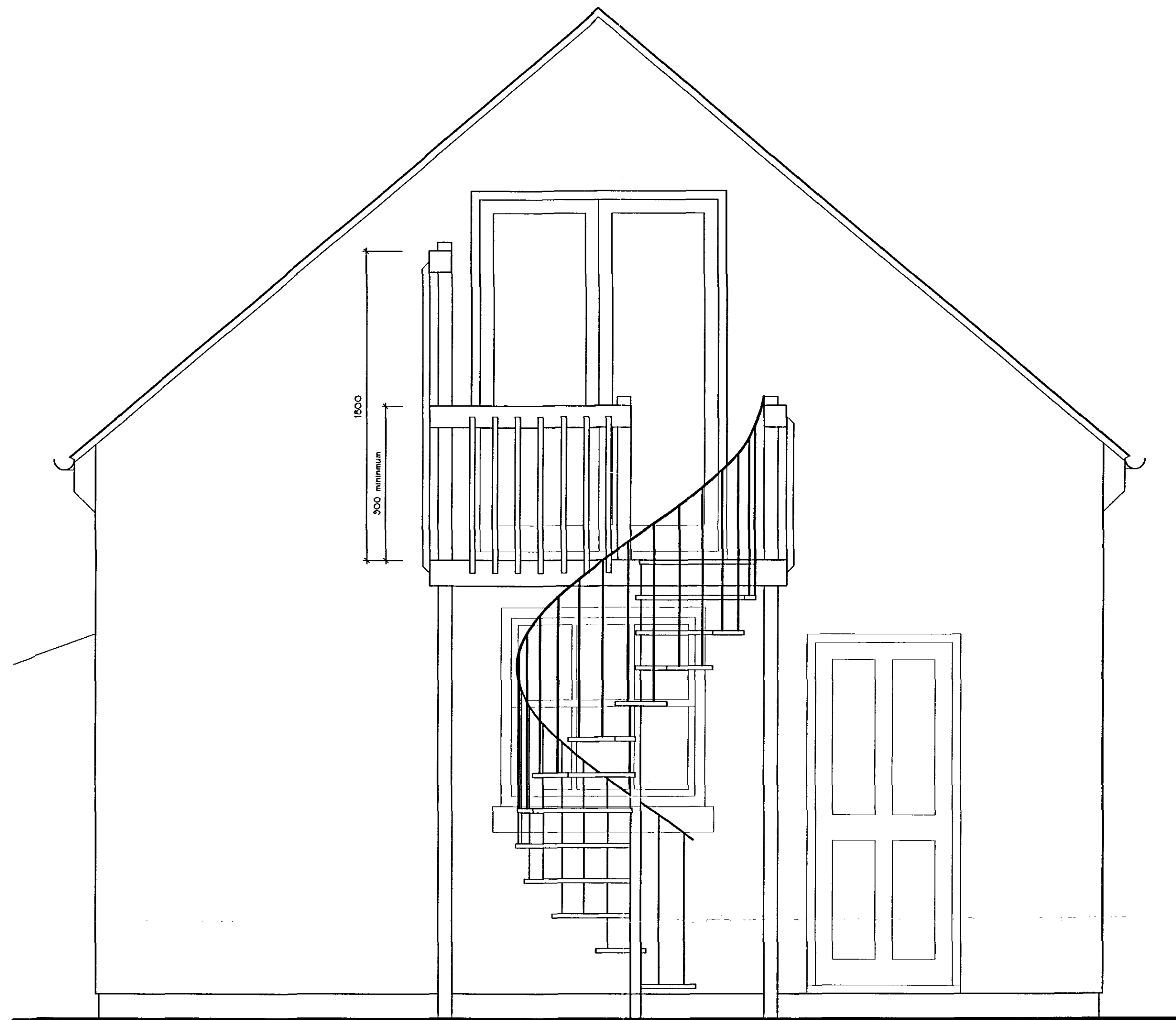
BALCONY SOUTH ELEVATION 1:20
