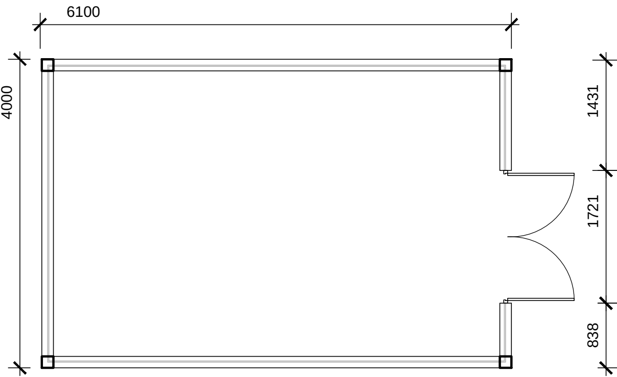
GLASS HOUSE ~ FLOOR PLAN SCALE: 1:50
