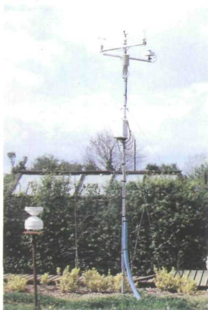
ABOVE: The site monitoring system collects data on local temperature and humidity.
