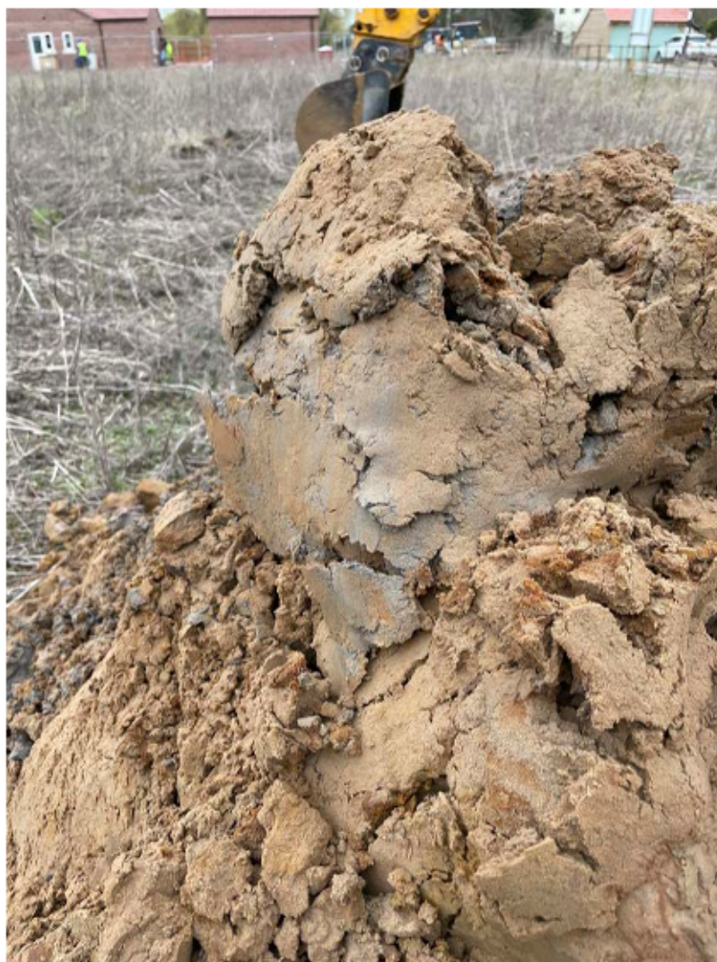
Image 7.0: SAND and silt, extracted from trial pit 4
