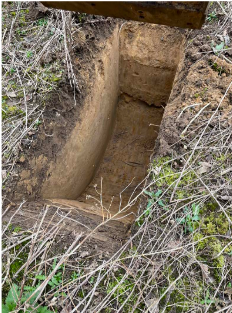
Image 1.0: Trial pit with 400mm topsoil, set at the head of a SILT bed.
