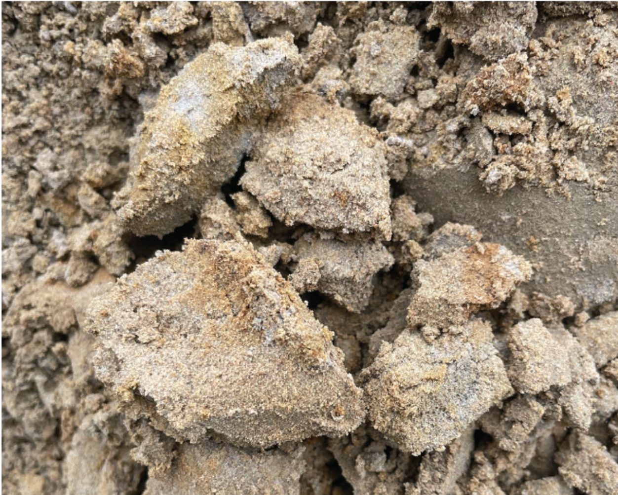
Image 2.0: SAND with SILT and mottling.
