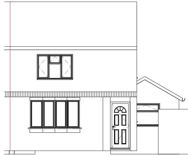
1 Front Elevation - (Existing) 1 : 100
