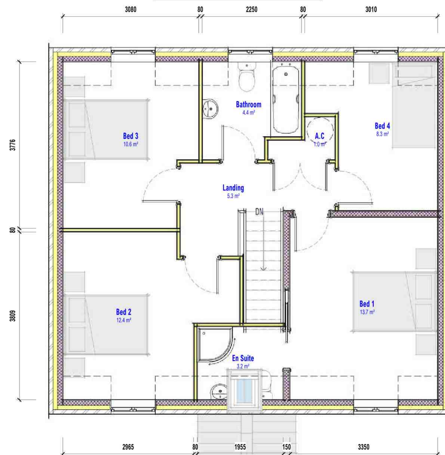
11 - Proposed First Floor Schedule Name Area Perimeter A.C 1.05 m 2 5.0 m Bathroom 4.35 m 2 12.3 m Bed 1 13.65 m 2 18.3 m Bed 2 12.35 m 2 19.0 m Bed 3 10.65 m 2 17.1 m Bed 4 8.30 m 2 16.1 m En Suite 3.25 m 2 7.2 m Landing 5.30 m 2 11.2 m Grand total: 8 58.85 m 2 106.3 m
