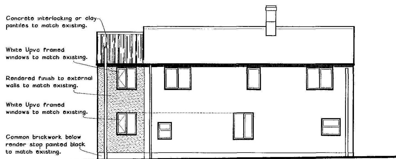
PROPOSED FRONT (NORTH) ELEVATION 1:100
