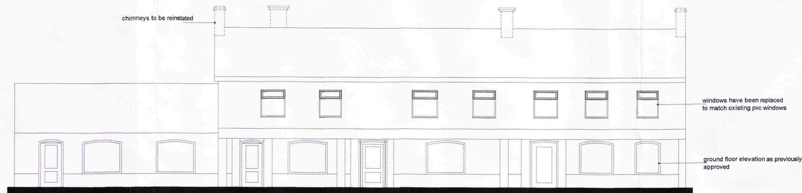
FRONT ELEVATION (north)
