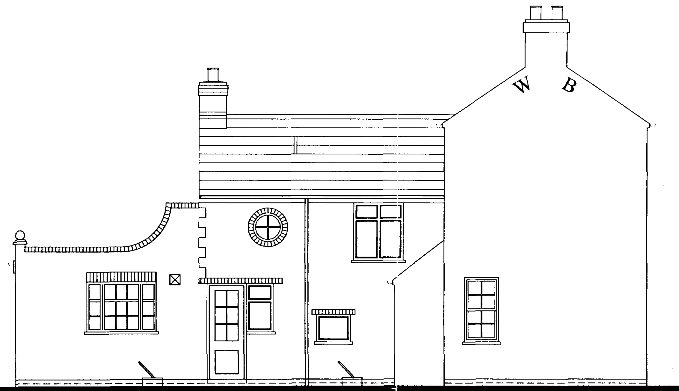
Elevation to Garden (West) as Existing Scale 1:50
