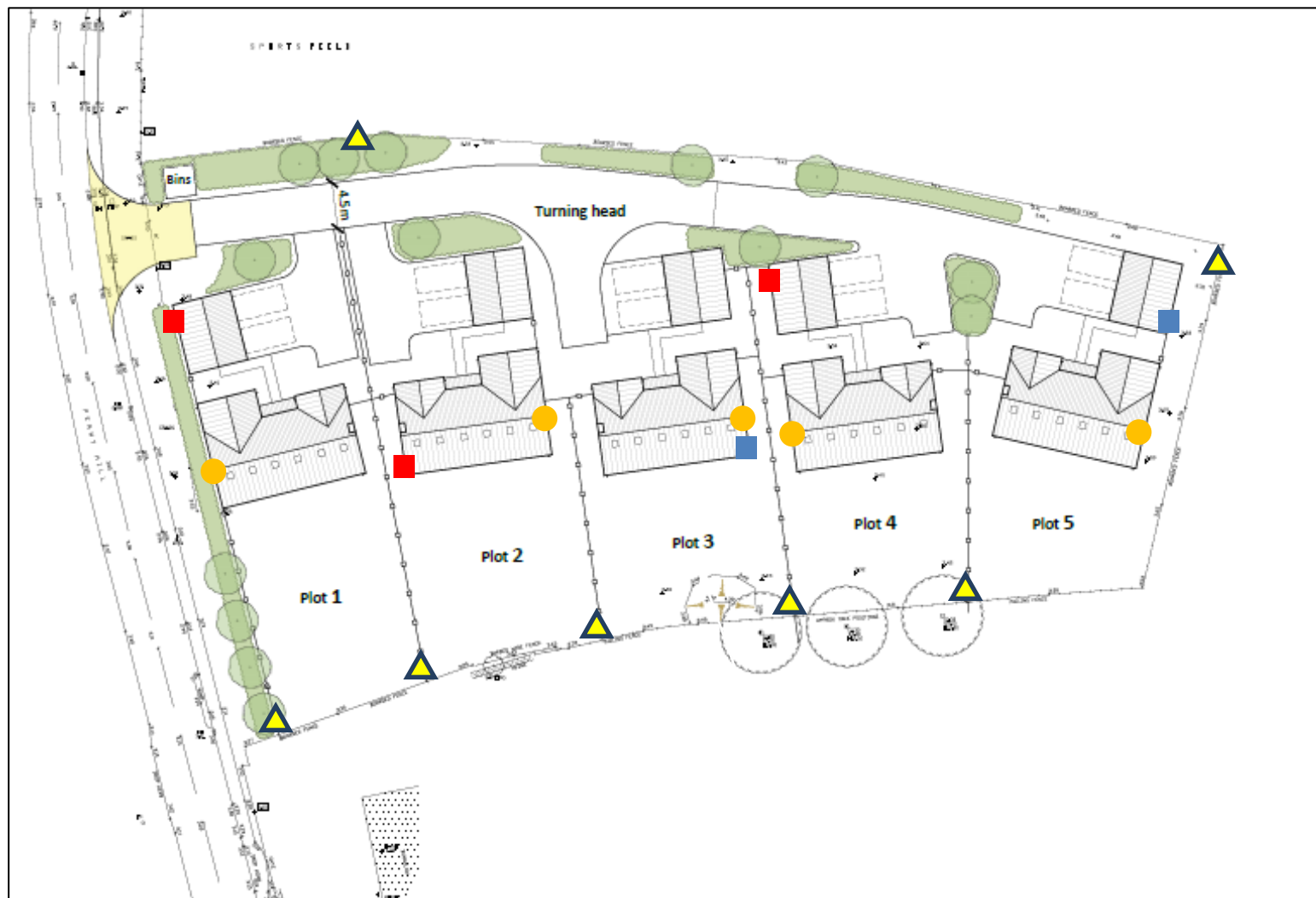
Figure 11. Location plan for installation of enhancement measures
