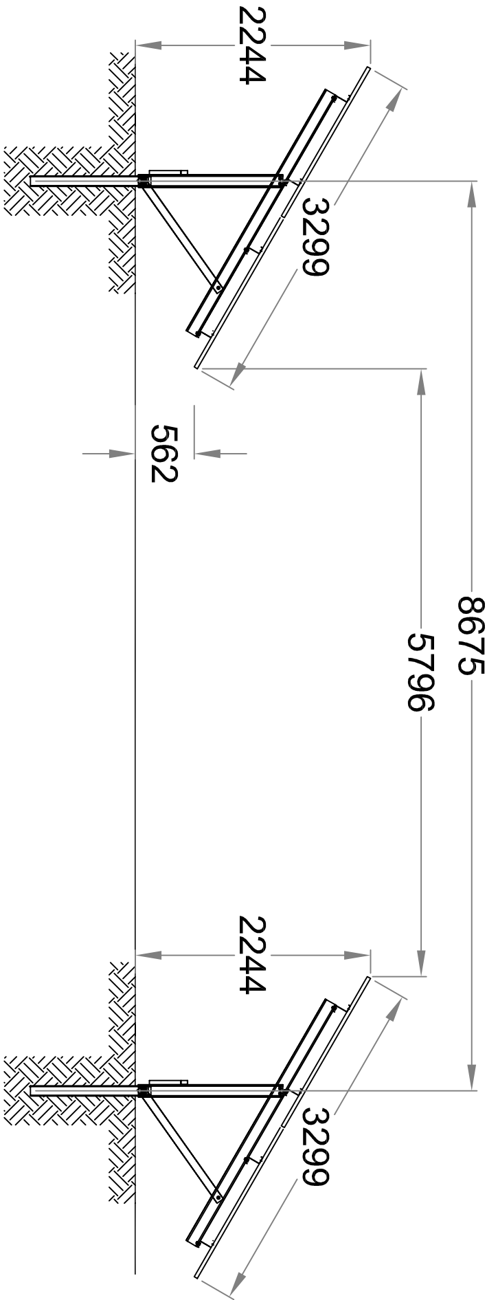
SIDE ELEVATIONAL VIEW (NTS)
