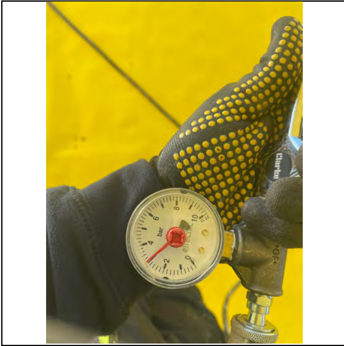
Air lance testing equipment.
