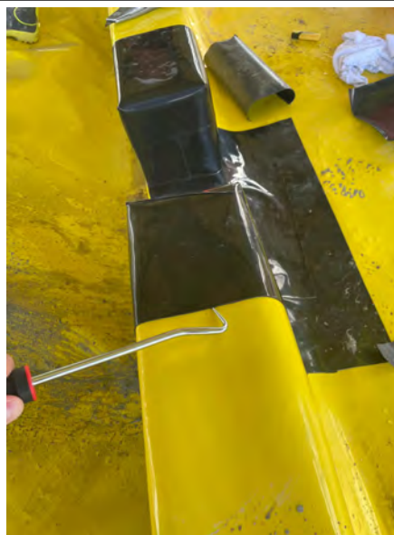
A pick and probe test being conducted upon the edge of a piece of Juta Titan Tank.
