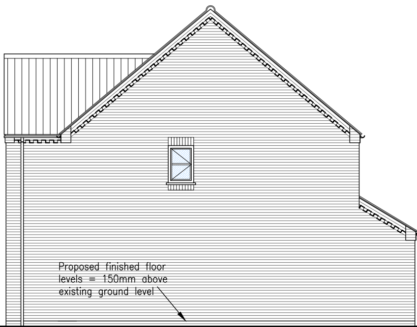
Proposed Side Elevation 1:100
