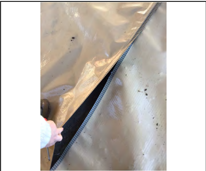
Fault found on welded lap
