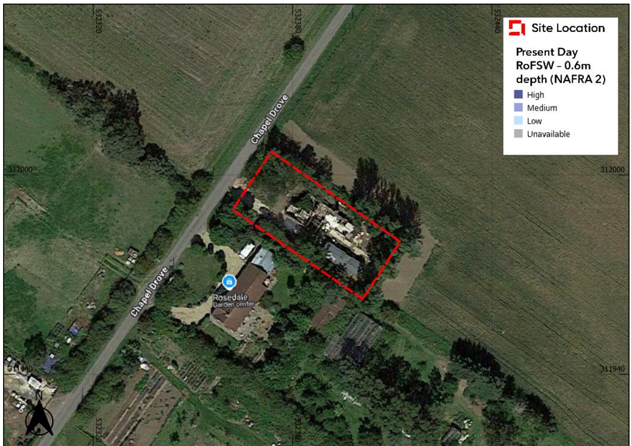
Figure 11: EA Surface Water Flood Risk Mapping Present Day Depth >0.6m (Base map and data from Google Hybrid © Contains public sector information licensed under the Open Government Licence v3.0)
