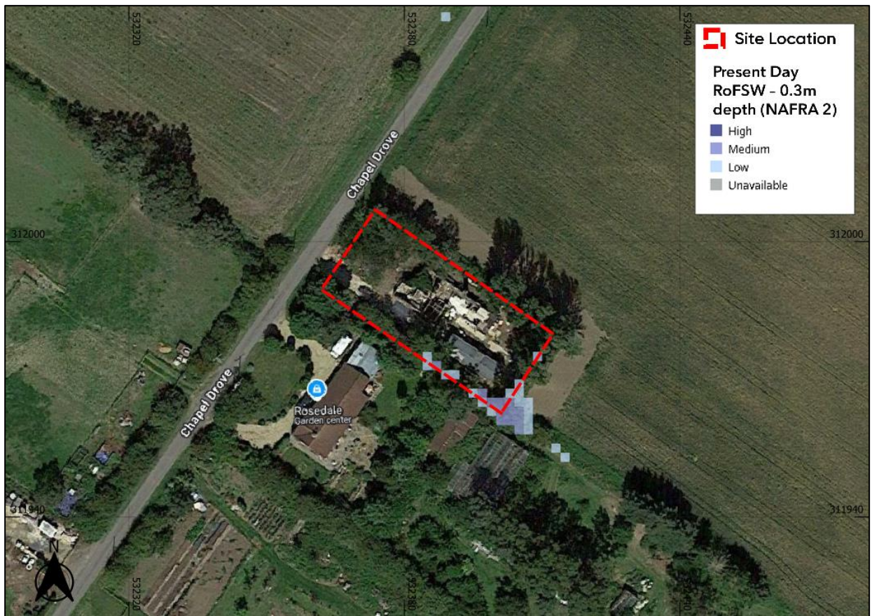
Figure 10: EA Surface Water Flood Risk Mapping Present Day Depth >0.3m (Base map and data from Google Hybrid © Contains public sector information licensed under the Open Government Licence v3.0)
