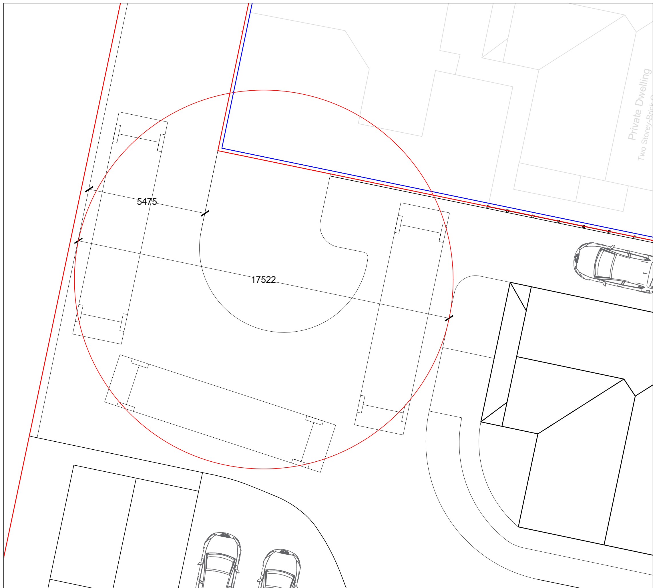
FIRE FIGHTING APPLIANCE TURNING FACILITY (1:100)
