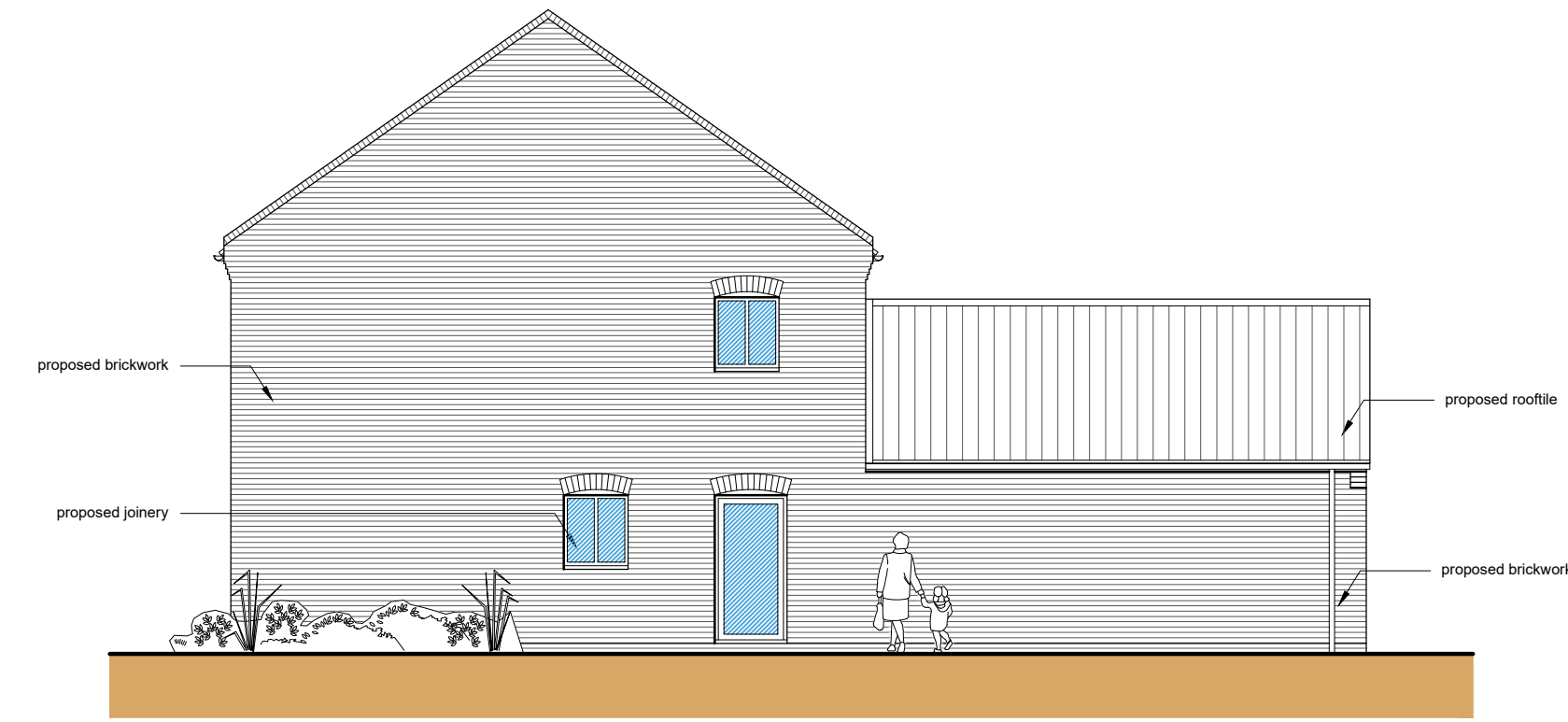
Side Elevation (SW) Scale: 1:100
