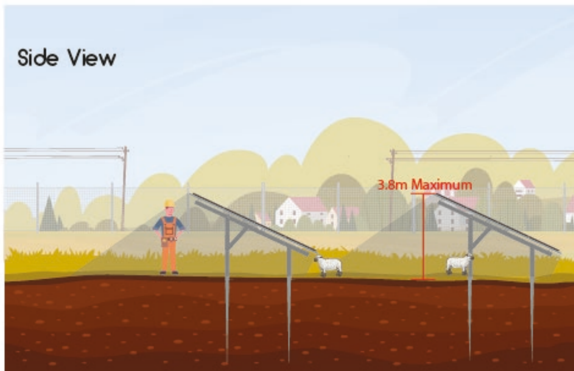
Typical Solar Panel Cross Section
