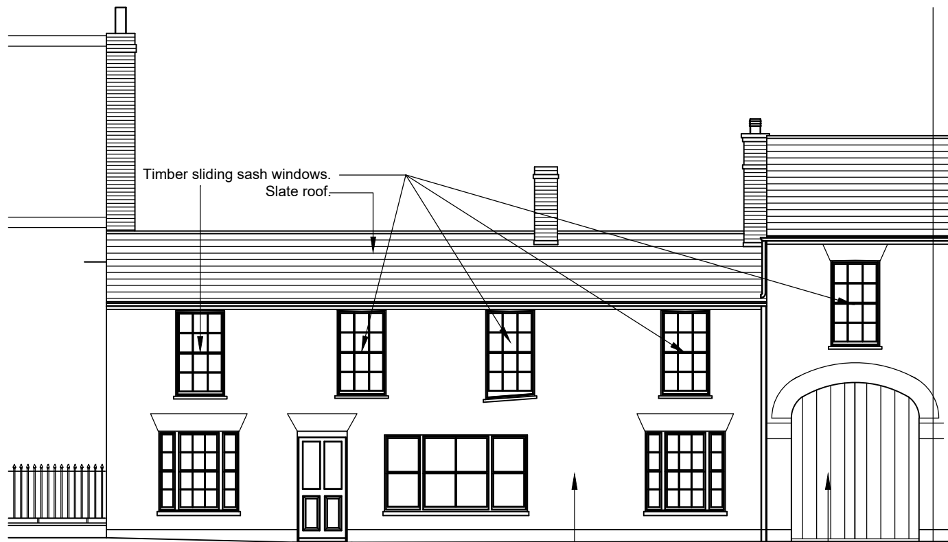
Elevation A - South Scale 1:100 Existing Elevations
