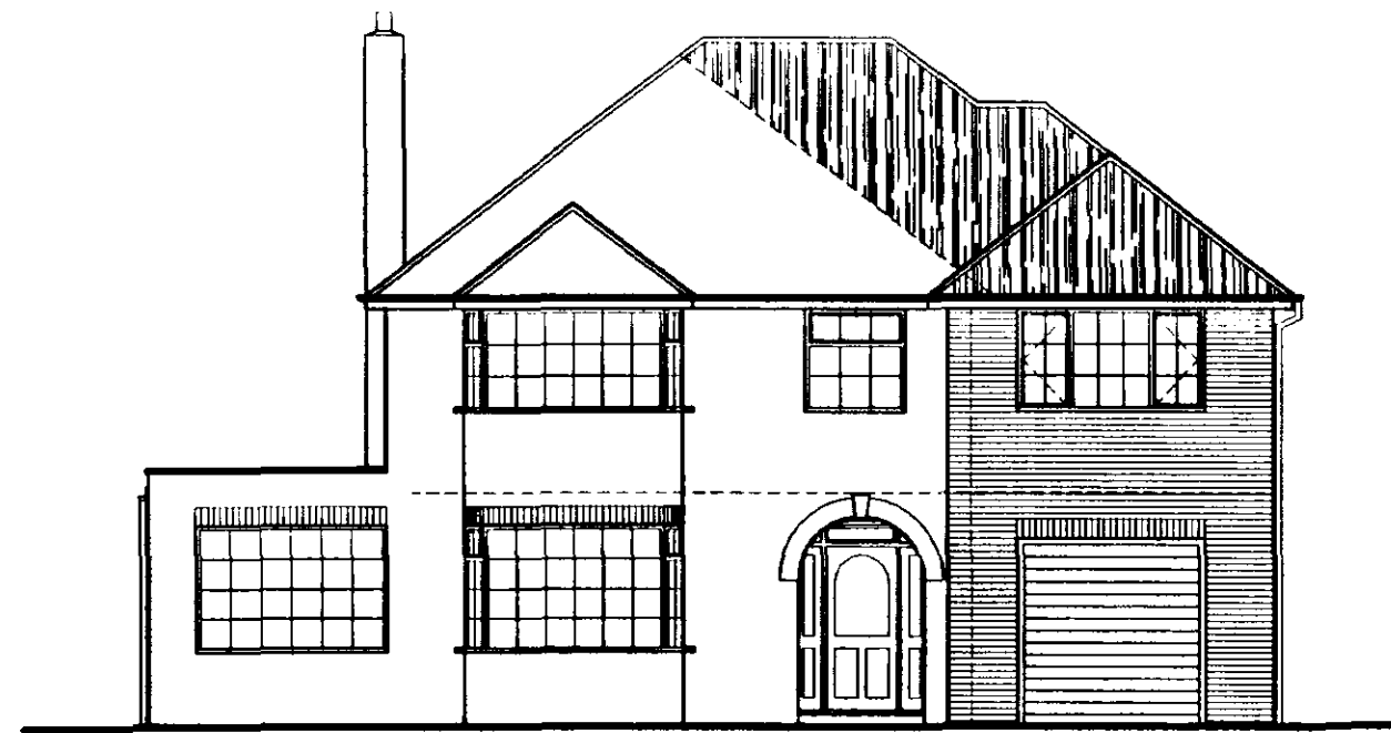
FRONT (EAST) ELEVATION 1:100
