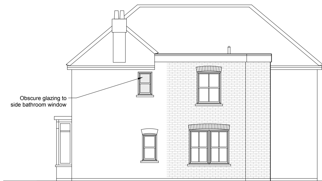
Side Elevation Elevations 1:100
