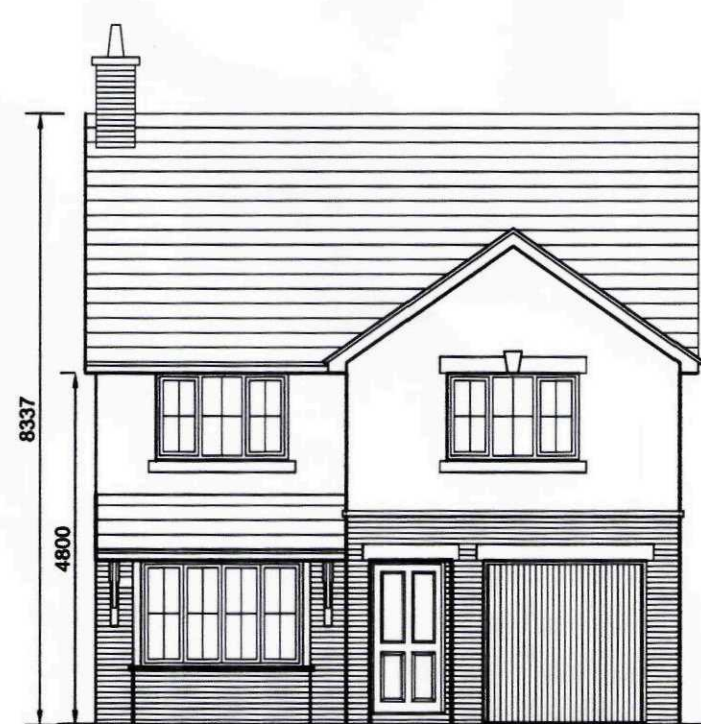
Front Elevation Plot 3, 50 & 74 plot 75 mirrored
