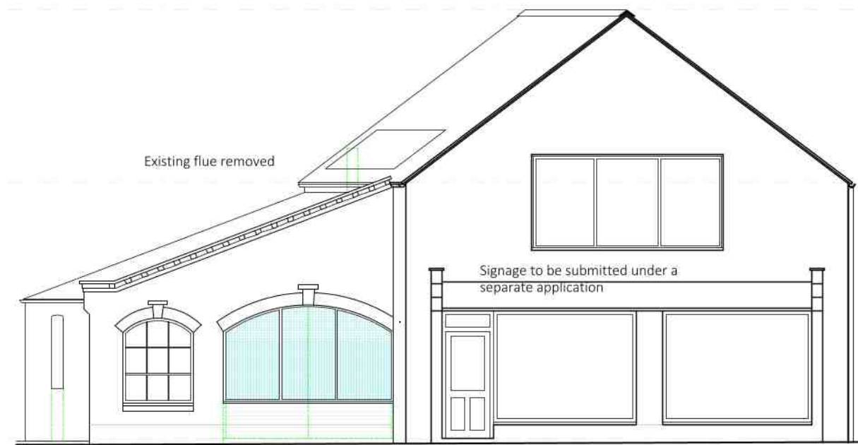
FRONT NORTH ELEVATION
