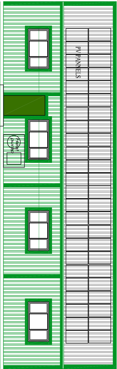
ROOF CLADDING GOOSE WING GREY PCS SHEETING
