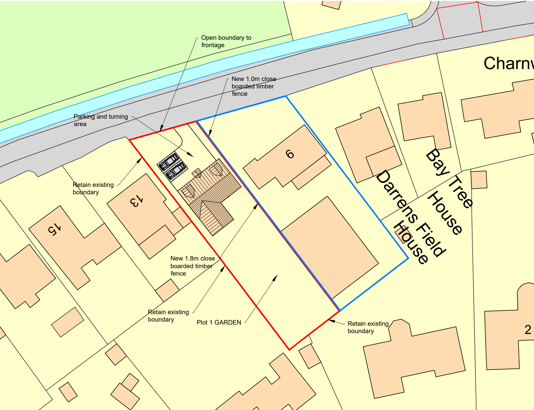
INDICATIVE BLOCK PLAN AS PROPOSED SCALE 1/500 @ A3
