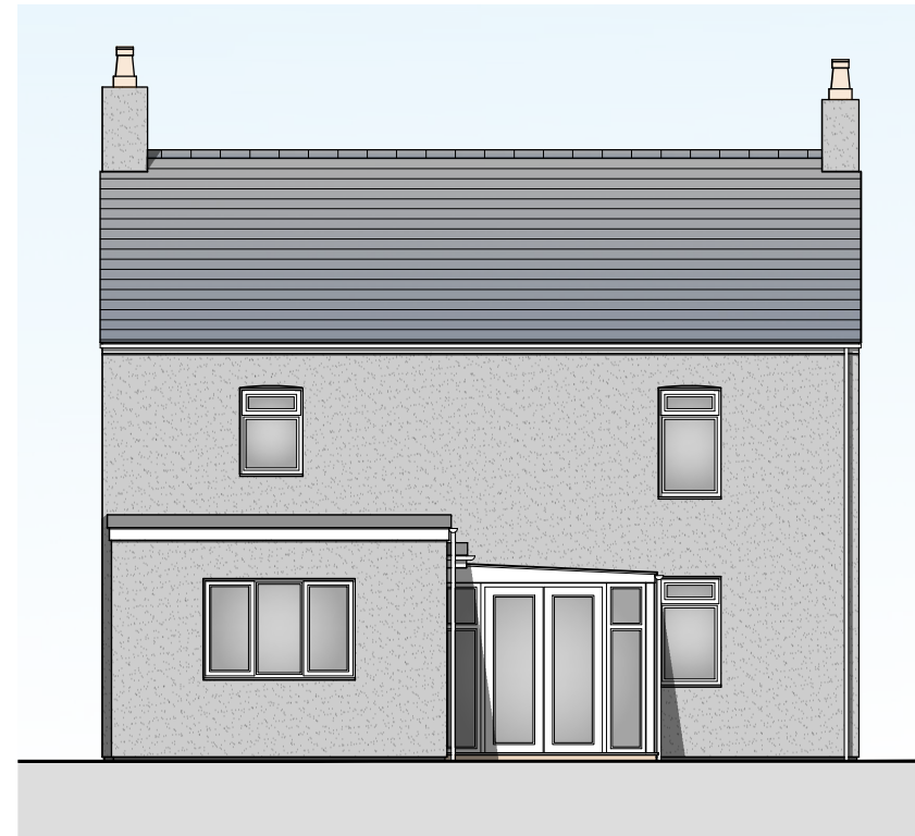
Proposed Rear (SW) Elevation Scale 1:100
